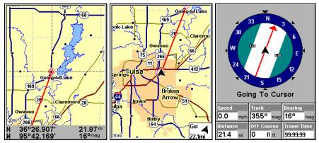
The first figure (left) clearly shows the red course line connecting your current position to your destination. The 30-mile zoom (center), shows both current position and direction to destination on screen. The Navigation Page (right) will also show navigation information.
